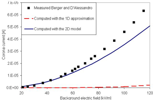
Figure 2. Comparison of the stationary corona current of a 1 m tall pencil-shaped rod computed according to the 1D approximation and with the 2D model. The measured values reported in [15] are also shown.
