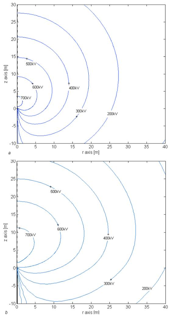
Figure 4. Contour plot of the shielding potential of the generated space charge produced by corona from a 60 m tall rod computed with a) the 2D model and b) the 1D approximation. The figures correspond to the results when the downward leader tip is 1200 m above ground
