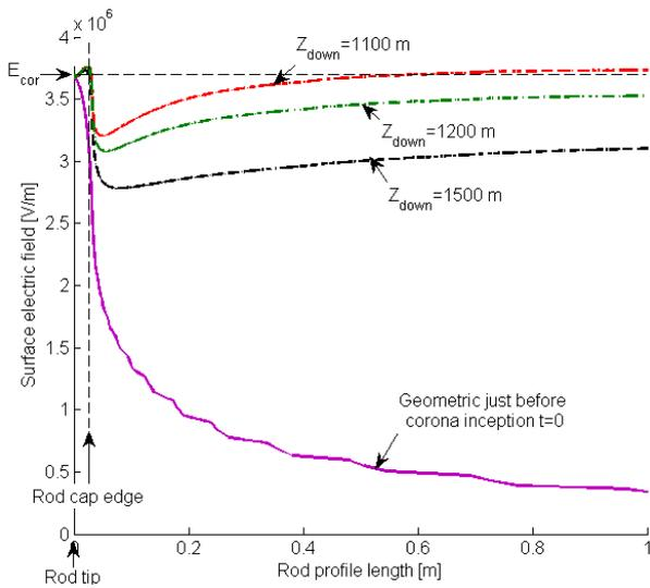
Figure 5. Electric field along the profile of a 60 m tall rod at different height of the downward leader tip.
