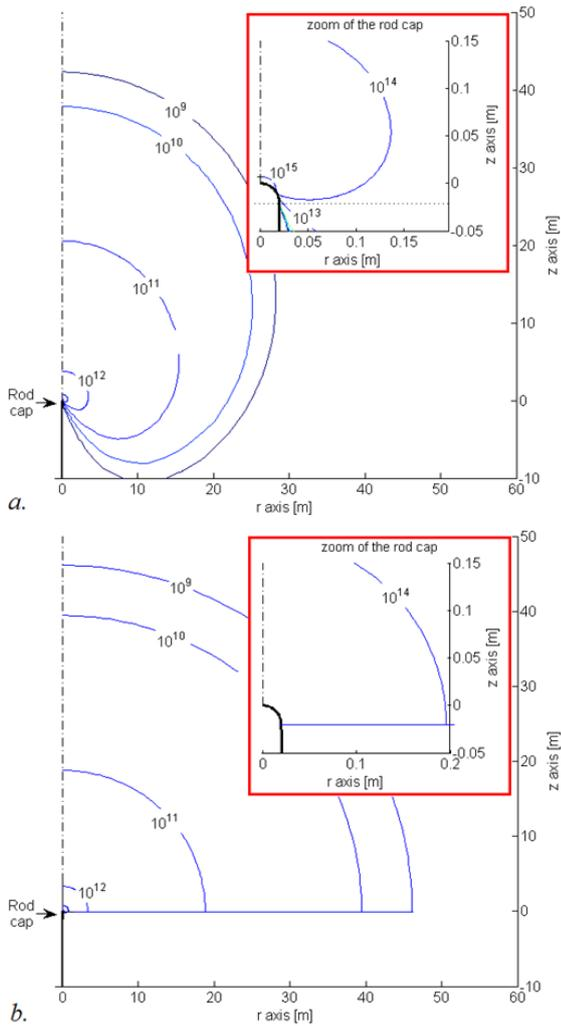
Figure 3. Contour plot of the small ion density produced by corona from a 60 m tall rod computed a) with the 2D model and b) with the 1D approximation. The results correspond to the electric field equal to 20 kV/m.
