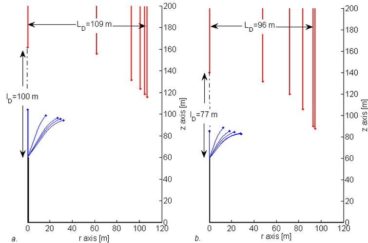
Figure 6. Simulated still photograph of the lightning attachment process for a 60 m tall, 0.02 m radius rod calculated a) neglecting and b) considering the glow corona space charge.
