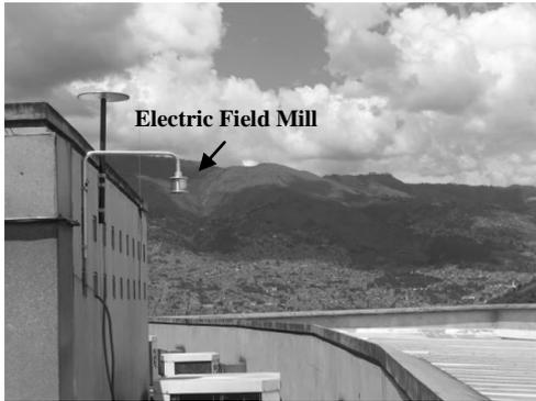
Figure 2. Electric Field Mill. (background: Non flat terrain and the City of Medellín)
