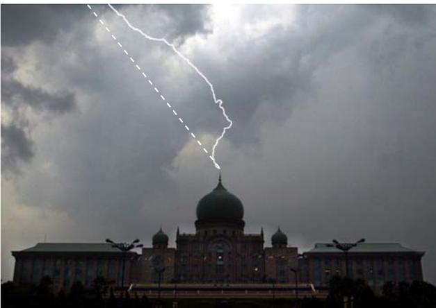
Fig. 9: The dotted line represents the hypothetical path of the early streamer according to the ESE hypothesis. (Photo credit: The Star Publications plc)
